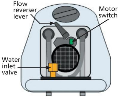
The flow reverser lever has two positions, LEFT, and RIGHT. If the lever is to the left, water will flow into the heating system through the left hand side hose, and water will return to the tank along the right hand hose. Pushing the lever to the right reverses the direction of flow and return.
