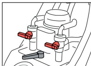
Position the unit in a room with a suitable drain point and a mains water supply. Set both isolation valves to the closed position. Run the drain hose and overflow hose to a suitable drain.
