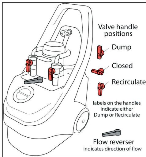
When 'dumping', the water level in the tank will fall as dirty water is diverted down the drain, and does not return into the pump tank.
